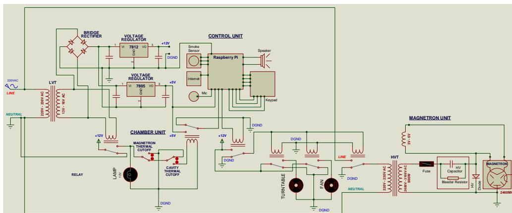
Command can be received either by keypad input or voice input. If voice input is used, Internet should be turned on. As soon as the command is received and recognized, the relays switches and the supply is turned on for magnetron and chamber unit. Apart from this, the door latch act as circuit breaker here, this means, if the door is open during or before operation, the microwave cooking will not process. This mechanism is just identical to the traditional microwave oven.
