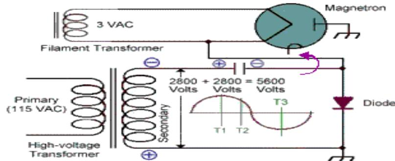
When the magnetron unit gets powered, the high voltage transformer produces 2800V, but this is just not enough to efficiently power the magnetron. Hence, high voltage capacitor and diode circuit is used which act as a voltage doubler circuit. The use of this circuit is to double the applied voltage and produce 5600V which should be applied to the magnetron cathode for the production of microwaves.
